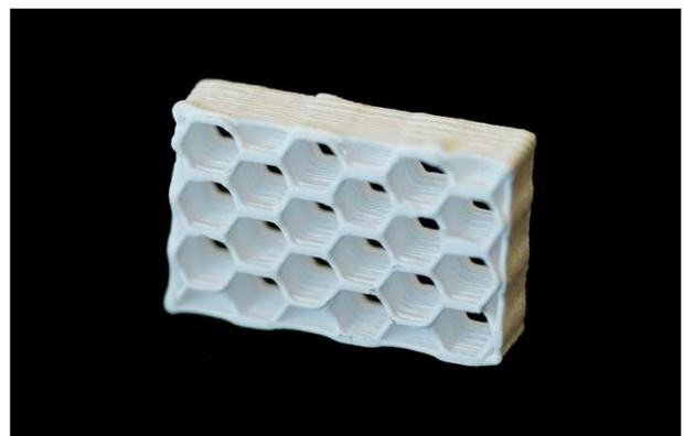
Al<sub>2</sub>O<sub>3</sub>-Keramik-3D-Druck, BxHxT: 30x17x5 mm
