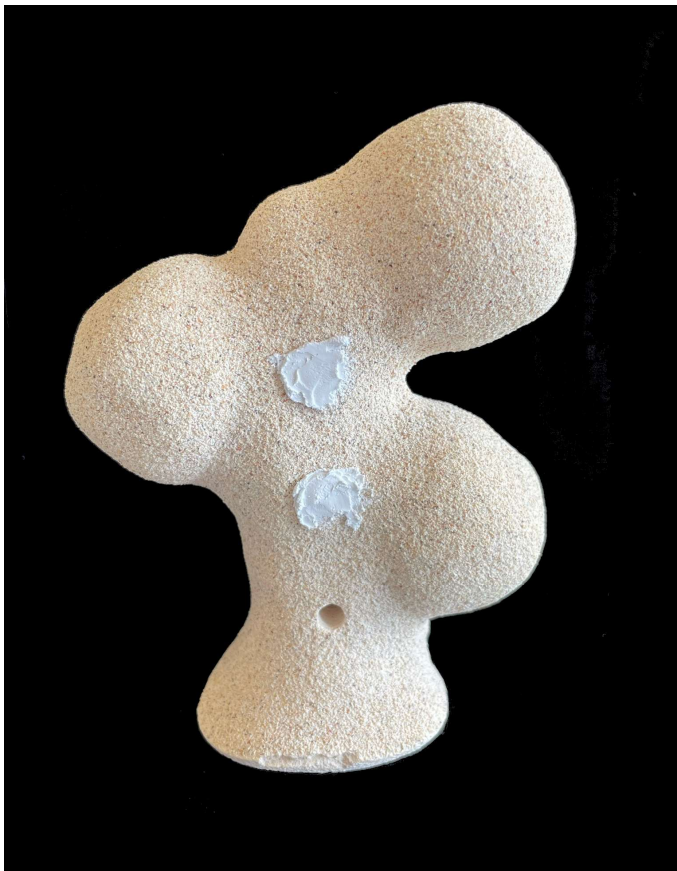
Fixed ceramic shell with FastCast slurry, HxW : 14x11 cm
